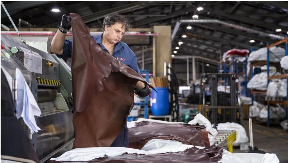
A worker prepares leather for vacuum drying at Packers Leather Tannery at Narangba. Picture Lachie Millard
